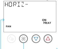
Press the warmer (up) and cooler (down) buttons to toggle the heat mode horizontal swing off and on.
