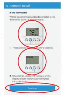
4. Press the fan button for 5 seconds to put the thermostat in "WIRELSS SETUP", then select "Continue".
