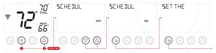
Press and hold the fan and warmer (up) buttons for 2 seconds to enter schedule mode for programming a schedule. While in schedule mode, press the mode button to advance through each setting for each day of the week and each time period of each day.
