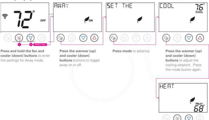
Press the warmer (up) and cooler (down) buttons to adjust the heating setpoint.
