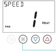
Press the warmer (up) and cooler (down) buttons to cycles through available fan speeds of auto and 1 (low) through 5 (high).
