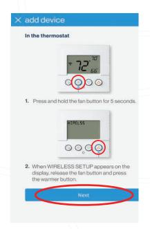
2. Press and hold the fan button on the thermostat for 5 seconds to put the thermostat in "Wireless Setup" mode.
